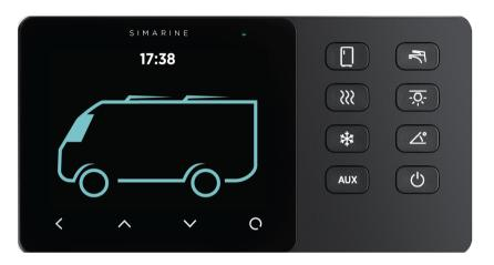
After the first power-on, there are no batteries and tanks displayed. Long press the 🖸 button to enter the settings menu.
