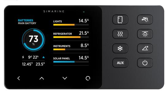
If the battery connects only to a voltage sensor (without a current sensor), the battery name, approximate state-of-charge (SOC), and current-voltage are displayed. The calculation of SOC takes some time, so it may not be shown immediately after power-on.
