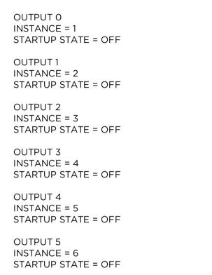
The default mapping instance properties of the outputs (RELAYS) is therefore:
