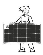
The panel can be supported by the edge but only by keeping it vertical and without exerting excessive pressure on the cells.
