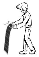
The panels should not be gripped by the ends and especially by the corners, to prevent them from flexing too much under their own weight.
